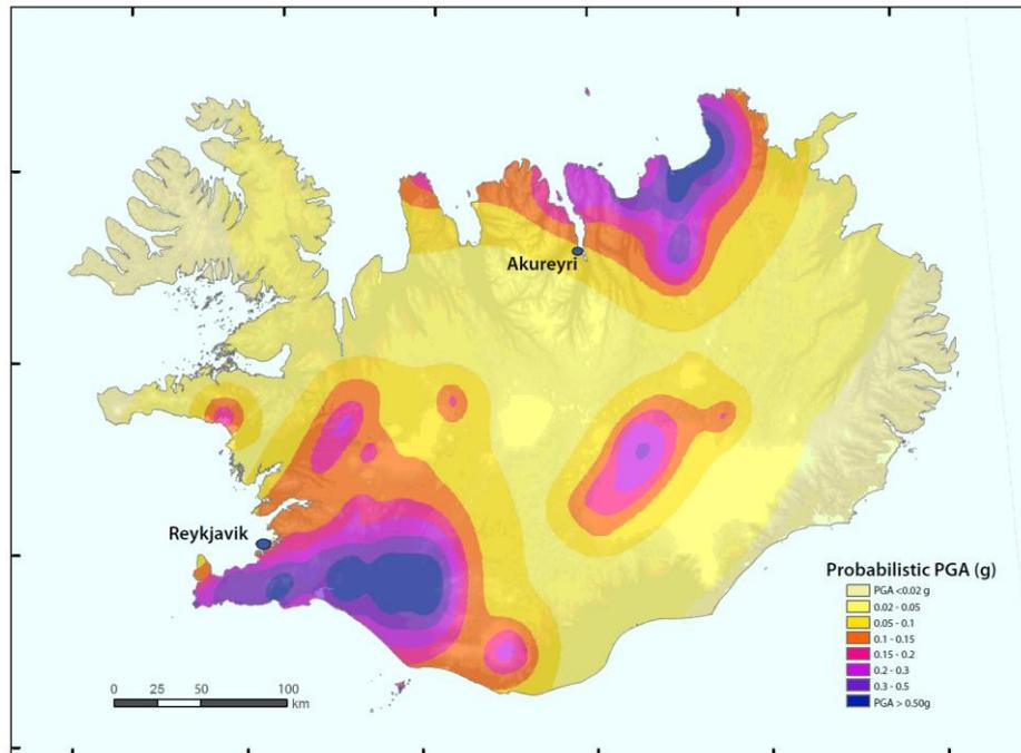
Figure 3. The Zolfaghari seismic risk map, which has been converted to portray the probabilistic maximum peak acceleration with a 475 year recurrence period.
