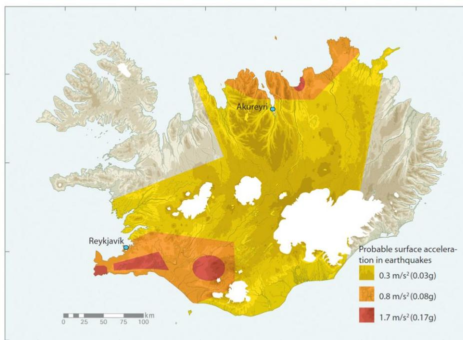
Figure 2. An earthquake hazard map proposal, showing probable maximum surface design accelerations, submitted by the Earthquake Hazard Commission 1958. No measured surface accelerations in earthquakes had been obtained in any Icelandic earthquakes at that time.
