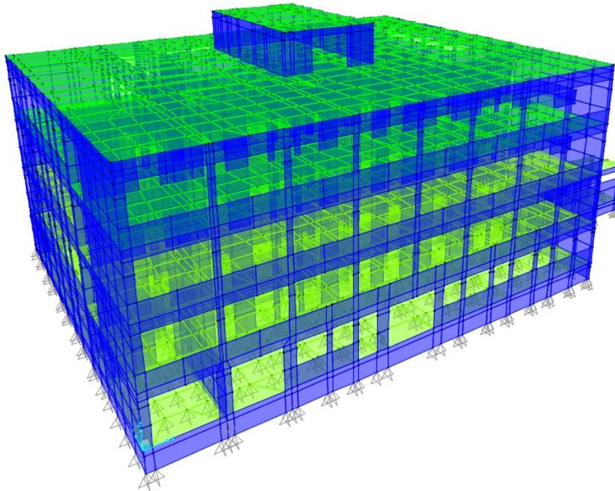
Figure 2. 3D model of the building in SAP2000
