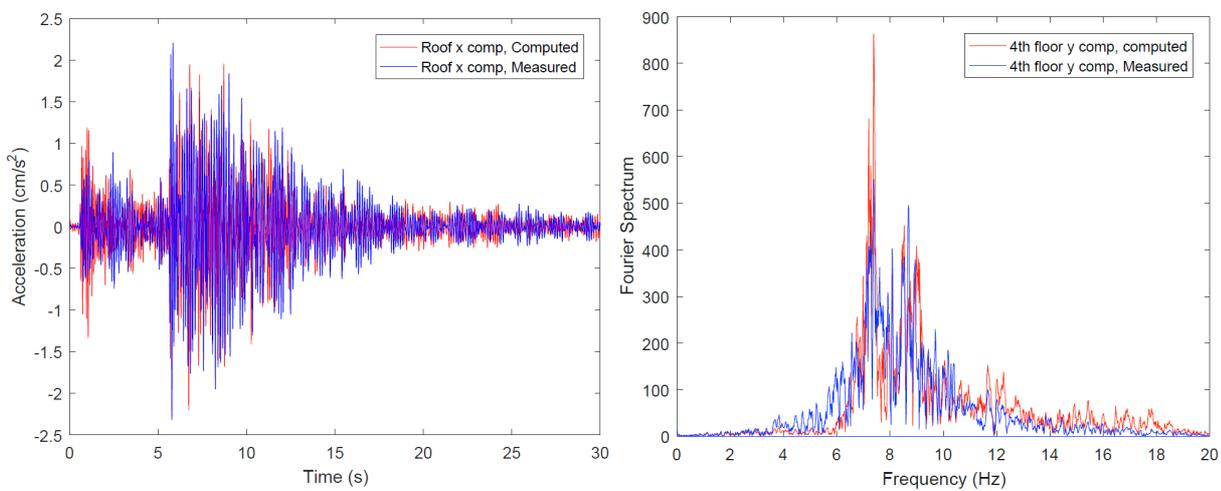
Figure 3. Comparison of recorded and computed response. To the left: Time series from the sensor within the utility building on the roof. To the right: Fourier spectra from the sensor at the top corner of the outer wall on the 4th floor on the right.
