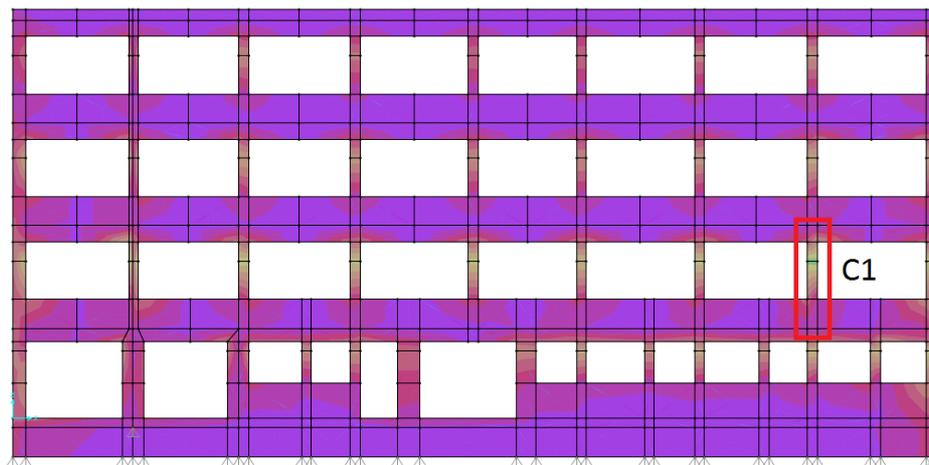
Figure 4. Vertical design forces in the south west wall of the building for a specific load case. The short window column at C1 is a cross section selected for further checking.
