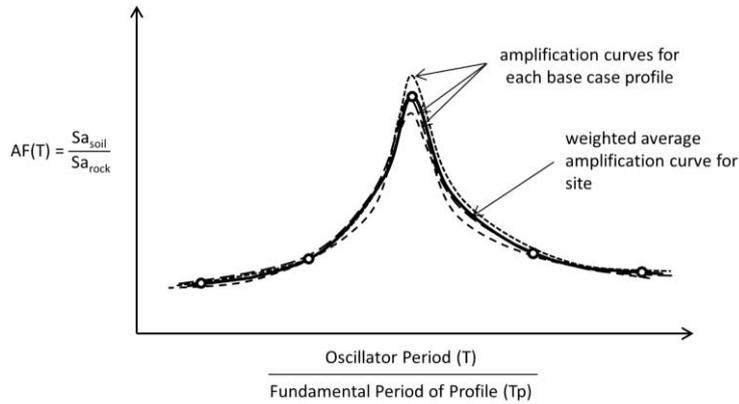
Figure 2. Amplification curves for each base case profiles expressed as function of the ratio of oscillator period to fundamental period of the soil profiles. The resulting weighted average amplification curve has both a bandwidth and amplitude that are statistically representative of curves for the base case profiles.
