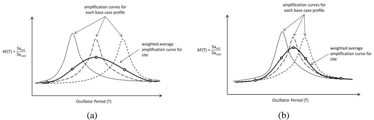
Figure 1. Amplification curves for each base case profiles and weighted average amplification curve for: (a) large assumed epistemic uncertainty, and (b) small epistemic uncertainty. The bandwidths of both weighted average amplification curves are greater than those for the base case profiles, and the amplitude of the weighted average curve for small epistemic uncertainty exceeds that for larger epistemic uncertainty over a range of oscillator periods.
